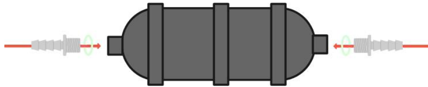
Figure 7 - Serrer les raccords de tuyaux
