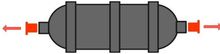
Figure 6 - Removing the seal caps
