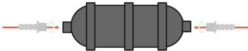
Figure 7 - Tightening Hose Connections
