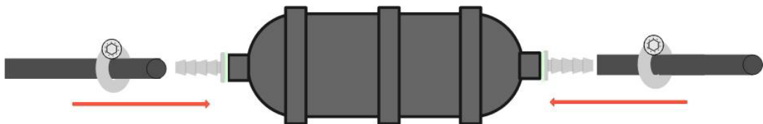
Figure 8 - Connecting the hose ends to the SGI filter
